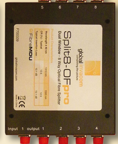
■ Globallnvacom modified the optical splitter with connector jacks: the optical connection cables can now be directly plugged into the splitter.
