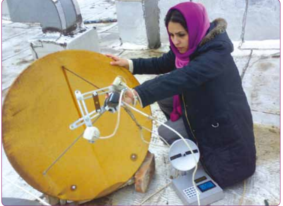
■ This is how the intelligent satellite finder is used: it shows the position of the satellites that are to be received and the real antenna is simply placed parallel to it.
