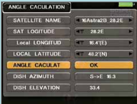
The Angle calculation simplifies the installation of an antenna
