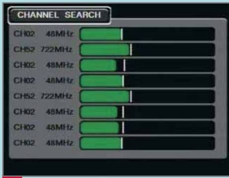
Multi Channel Search for DVB-T lets you view 8 channels Signal Quality simultaneously |
