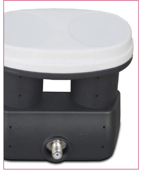
The holes at bottom of Monoblock keep it dry inside, allowing for condensed water to leak out
